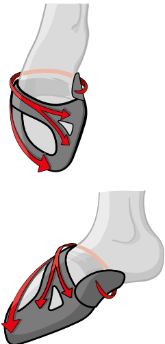
PRESSURE DISTRIBUTION OF 3-FORCE SYSTEM
